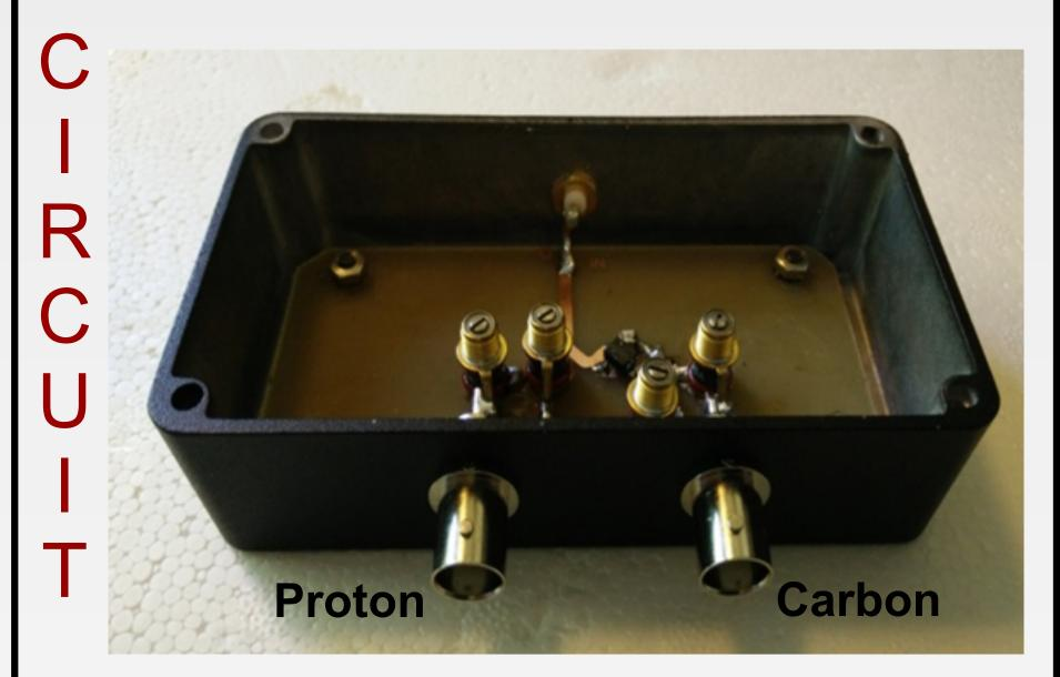
The tuning range for both channels is  $\pm 3$  MHz. Simulated and measured S11 is approximately - 45 dB and -55 dB for at carbon and proton frequency, respectively. Measured/simulated Q factor of the whole system at 285.5 MHz is 76/104 and 71.8 MHz is 38/50.
